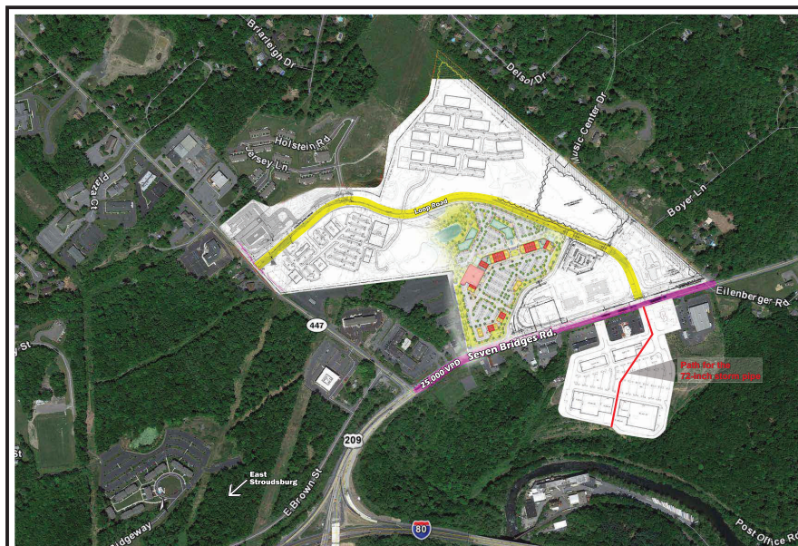
A drainage pipe extending south of U.S. Route 209, as show in red, will carry stormwater from Smithfield Gateway to Brodhead Creek. [PHOTO PROVIDED]
